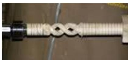
Stuart showed how the bines can be roughed out and shaped using a small saw, carpenter's chisel, rasps, Arbortech, etc. Finishing as always was with Stuart's "special tool" (twisted strips of abrasive paper to you and me).
