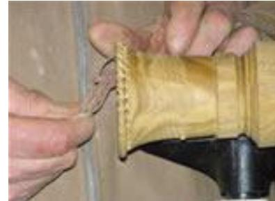
drilling through a small hole (32 times) to allow the ribbon twist to continue around the rim before shaping and sanding.
