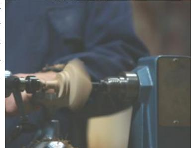
The spigot diameter was reduced so that it would fit between the chuck base plates (not the jaws), but also forming two larger diameter spigots to sit on the jaw face. The piece was reversed, the bottom of the bowl shaped and the inner sides of the three feet reduced to produce consistent edge thickness.
