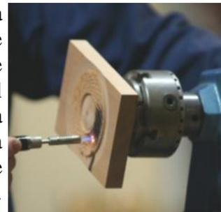
Scorching in the centre and around the edges was cleaned up with a gouge.
