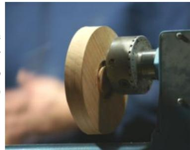
Two "V" shaped grooves were cut into the face of the disc, fairly deeply, using a skew chisel held horizontally on the rest and used as a shear scraper. These circles are reduced to arcs when the disc is thinned, and are probably the most difficult cuts to make in this project.
