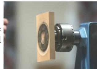
The plaque was remounted on a second screw position and a groove about 1 cm wide was cut using a parting tool. Due to the position of the groove part of the ebonised section was removed and part was "off the edge". Additional grooves can be cut to create a concentric off centre pattern. Simple but very effective.
