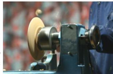
A specially made mounting board was used to reverse mount the disc. This was a circular plate with a spigot on the reverse for mounting in the chuck. The face had been cut into a concave shape with approximately the same curvature as the face of the project disc. Using a piece of router matting the disc was clamped between the plate and tailstock. The router matting was placed between the plate and the disc, and care was taken to mount the disc as centrally as possible.
