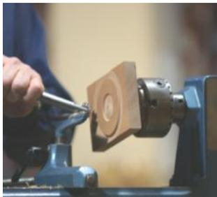
The blank was mounted centrally and a raised circle was cut, with the centre of the circle reduced and the remainder of the face thinned out to the edges. A spiralling tool was used on the raised portion to create a surface pattern, which was ebonised with a small butane torch, making sure that the scorching went into the deep grooves.
