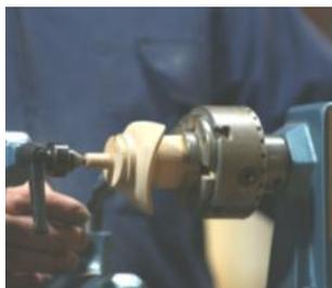
The bowl was removed and a small cylinder was mounted in the chuck. This cylinder had a concave face, fitting the base of the bowl which was then mounted between this and the tailstock. The spigots were turned away with the centre spigot being reduced to a small diameter.
