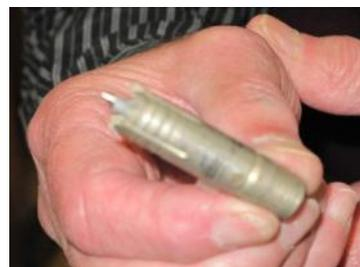
A circular cutter, made from a tin opener cutter and bar, and a scraper which uses a metal work square cutter were also shown, as in these photographs. Again, fairly simple to do, but a tap and die set would be needed. (I bought a set from Aldi for about £7.00 a few months ago.)
