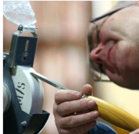
The jig attached to the grinder platform was used, with adapter for skews fitted. Greg was able to set the leg distance for the jig by sighting the angle of the bevel on the wheel and adjusting until “flat” against the wheel. One “trick” is to use a marker pen on the bevel and when the chisel is resting on the wheel, hand rotating the wheel and checking to see if all of the ink has been removed, and adjusting the jig leg if necessary.
