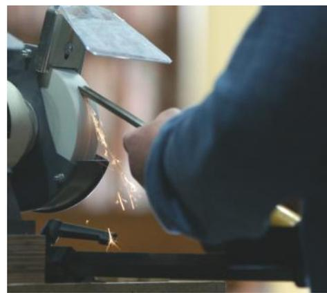
Greg went on to show how to create a longer grind, by removing the wings using a “rolling” action across the face of the wheel. He did point out that it was very easy to end up with a “bird’s beak” when creating this grind, which is countered by starting from the wings and then blending to the centre of the chisel, rather than profiling the middle and working outwards.
