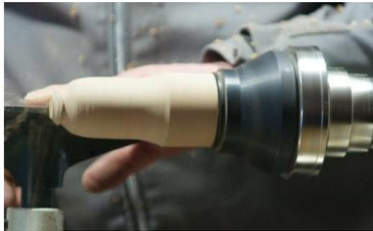
When the shaping was completed, the surface was sanded and a friction polish applied. At this point there was a discussion about the merits of using paper or cloth as a buffing medium with some members preferring the relative safety of paper and others preferring the possibility of a higher gloss with cloth.
