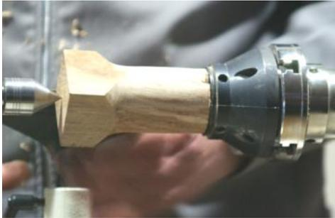
Having roughed a blank to a cylinder, involving reversing to blank to remove the residual square end, Malcolm shaped the “sharp” end, whilst starting to turn down the diameter at the headstock end. Most of this work was achieved using a skew to create the curves required.
