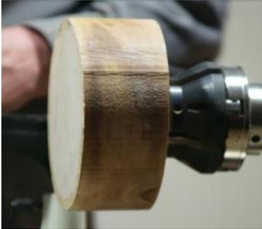
Having secured the screw chuck base plate into the O'Donnell jaws (not seen that before), the blank was roughed into a cylinder. Using a number of chisels, which were not as sharp as Malcolm would have liked, the external O.G. was formed, with a good surface leaving very little sanding requirement. A chucking point, which could become a foot, was turned onto the base, and the bowl was supported by the tailstock during this part of the project.
