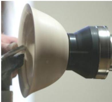
After reversing the bowl, the centre was hollowed using a 1/2" gouge, working down until a reasonable wall thickness was achieved.
