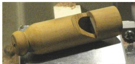
cut a flat on it, which was about ten millimetres wide. He inserted this into the end as far as the first saw cut and glued it in place. When the glue had set, he cut the insert off flush with the end of the whistle and made another slanting saw cut to form the mouthpiece of the whistle. The wall thickness was then reduced to about four millimetres by turning and shaping the outside before finally parting it off. The whistle was very effective giving out a high shrill note.
