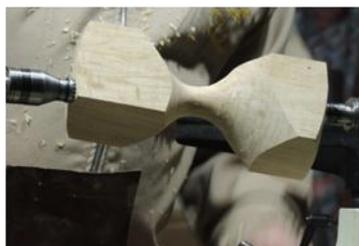
The second project was a LED illuminated Christmas decoration made from lime as a light (in weight) timber. The main globe was made from a piece 3 inch square by 3 1/2 inches long, which was turned round and a chucking point added, then mounted in a chuck. His method of hand turning a sphere
