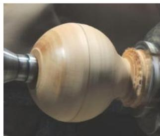
was to mark the centre, making an allowance for the top having a flat, then marking a couple of points 42% of the diameter, about the centre. He used these lines to cut off the corners at 45 degrees finally rounding the sphere by hand. The inside of the sphere was removed with a spindle gouge and finally finished to a 4 mm wall with a round shear scrapper. He made his own tips from 1 inch Silver steel bar drilled and parted off as a thin disk and
