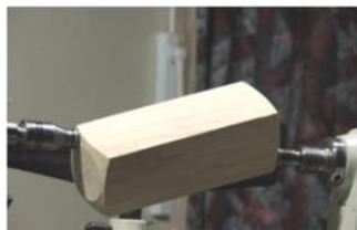
He started with the first of 3 off-centre candle sticks. This one, nicknamed his 'Dog bone' style, was made from a 3 inch square by 8 inch blank of spalted sycamore. It was prepared with a counter bore in one end for a candle sconce and placed between centres. All he did, whilst between centres, was trim each end at about 10 degrees. He then
