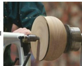
He turned the top edge with an internal rim which the lid would rest on. He then hollowed out the interior of the vessel using a long handled bowl gouge, by using this he was able to make very heavy cuts and removed the wood from inside of the bowl very quickly. His bowl gouge had a double bevel to allow him to cut tighter curves and for the final shaping he used a square tipped gouge. He finished the inside by using a scraper.
