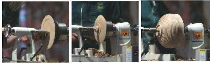
Mark discussed the type of foot that could be used. He demonstrated this by mounting a scrap piece of wood in the lathe, he quickly turned a foot on it and by using a rotary cutter formed three feet.
