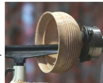
The lid was then held by pressure from the tailstock against a scrap piece of wood, held in the chuck. The lid was turned to size and a knob shaped on it. The bowl was then reversed and held between a friction pad and the tailstock whilst the foot was turned.
