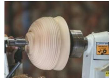
He then reversed the bowl on the lathe holding it in the jaws of the chuck (after removing the drive centre) preparatory to coring out the inside of the bowl to use as the lid. He discussed coring tools and said that normal parting tools should not be used as they are not strong enough and could twist and jam with disastrous consequences. He started coring out at a point slightly below the rim of the bowl so that the cored out piece was the same diameter as the bowl.
