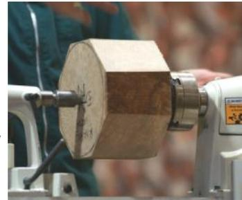
At the headstock end he turned a cove. Mark said that he wanted to put a series of beads on the vessel but getting the spacing right would be difficult by using a bowl gouge so he used a beading tool to create a continuous set of beads from the neck of the vessel to the base.
