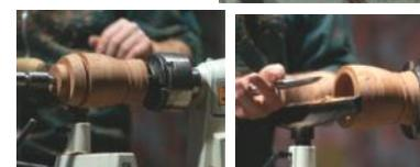
tion of the blank to form the lid. He then held the main body of the box in the chuck. He removed the inside of the box with a flat half-round tool. He removed the waste very quickly using heavy cuts. He fitted the lid in the chuck removed some of the waste from the inside of the lid and turned it to fit so that two pieces of paper were needed to hold the lid in place in the box. The box was held in the chuck and the lid fitted and the outside turned to shape. The lid was shaped and finished.
