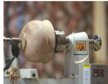
One wing of the beading tool had had the point ground so that a flat was formed between each bead. Mark then removed alternate beads from the bowl using a rounded scraper to produce an ogee shape between the beads.
