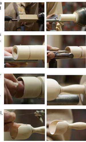
ing the handle came next followed by locking the lathe shaft so that the top part of the bowl could be sawn off to form the open scoop. The cut edges were then sanded to blend in with the rest. Finally, with the lathe unlocked, the finished scoop was parted off from the waste piece left in the chuck
