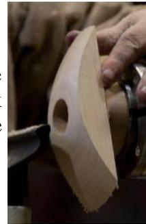
The outside was carefully turned into a curve and the piece reversed on the jam chuck. The inside curve was turned producing a curved stand for the egg box.
