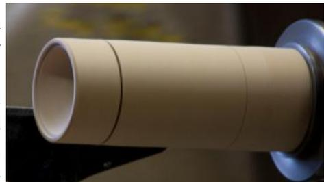
A register was turned into the lid and the outside turned into dome shape and parted off from the base.
