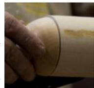
The outside of the base was then turned down so the box resembled an elongated egg. He then made the classic mistake of not checking the depth of the hollowing and cut through the wall.
