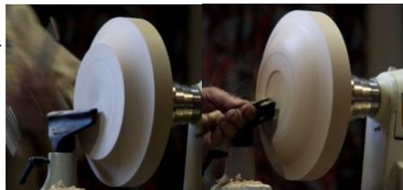
Tony then produced a large range of Sorby spiralling/texturing tools and proceeded to demonstrate how they were used on the underside of the platter. The tools were angled at different directions to achieve slightly different patterns. This was then sprayed black which I thought did nothing to improve the effect.
