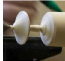
The second top had a ring of Corian added which added momentum to the top when spinning. The pre-drilled Corian was glued on to a spigot with superglue. The excess glue was set using activator but he still had the sense to stand to one side when the lathe was switched on.
