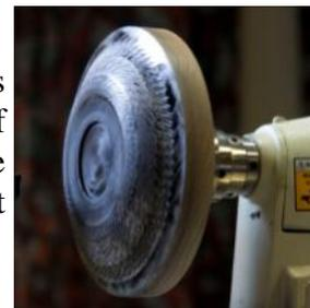
Reversing the blank, which was quite a bit thicker than needed, he commented that this could be used to practice different effects. The face was cleaned up with a gouge and then showed several methods of decorating the edge of the platter. Partly by using French curves and the airbrush, then using shapes cut out from artists 'Frisket'. Finally he finish turned the platter cum shallow bowl without any decoration.
