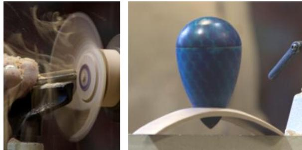
In the afternoon, Tony mounted a large roughly shaped piece of ash on to a screw chuck. He demonstrated the draw cut to flatten the front face by setting the gouge and then rocking his whole body backwards giving a flat surface.
