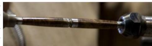
Since the blanks tapered in opposite directions Tony suggested all turners should be ambidextrous - easier said than done. The pen was sanded from 320 to 600 grit and then the surface was further improved using Micromesh up to 12000 grit. His preferred finish was two
