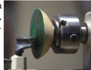
David uses the glass inserts that are available from a well know Swedish furniture company. He now shaped a recess for this insert in the top, so that the glass insert is flush with the wood (or protruding slightly, for safety reasons), and slightly wider than the insert, to give the wood a chance to move without breaking the insert.
