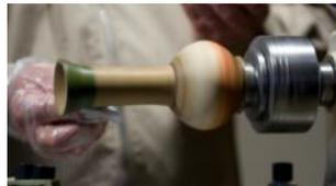
He demonstrated this on a pre-turned laburnum vase. It should be noted that the stained piece should not be sealed prior to staining, and care must be taken to use a sealer that uses a different thinner than the stain, otherwise the colours will get all messed up (i.e. spirit based stains should be sealed with acrylic sealer).
