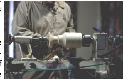
He then shaped the top of the vase with a bowl gouge. Once he was satisfied with the shape, he removed quite a lot of material from the waste section and then formed the bottom of the vase into an essentially hemispherical form. From there he then worked his way up towards the neck until he could blend the top of the sphere shape into the neck. The neck was turned down to 50mm, which left 5mm wall thickness once the core has been taken out with a 40mm Forstner bit.
