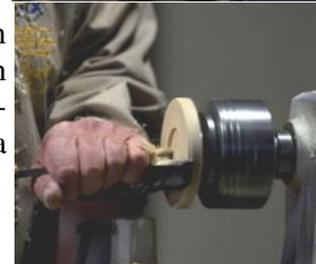
The lid, was reverse chucked to remove the tenon, and shaped into a slight dome. It was sanded to about 120grit and finished with cutting wax. This was repeated for the other lid and both were glued into place with medium CA.
