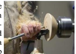
The blank was then chucked onto the recess in the bottom, and the face was trued up. He then shaped the top to a gentle curve falling to the 10mm line on the outside. This was again sanded to 400 grit. He then used a wire brush to remove the loose bits from the open grain (this technique works similarly well on other open grained woods, such as oak or elm).
