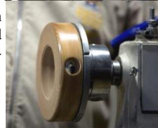
The two inserts to cover the opening in the centre were made from spalted beech. The first step was between centres, to create a tenon on one side. He then chucked it onto the tenon and shaped the outside to fit into the shoulder, and then created a chucking point with a parting tool. This can be compression or expansion fit.
