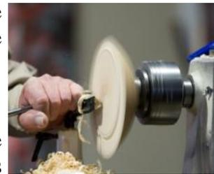
He then shaped the bowl, running at relatively low speed, as the piece is now severely unbalanced, and this worsened as more material was taken from the centre. The wide part of the rim is ideal for further decoration, e.g. pyrography or carving. The tenon at the bottom of the bowl has to be sanded off, as the bowl cannot be mounted the other way (the inside of the bowl is off centre and will prevent any proper mounting).
