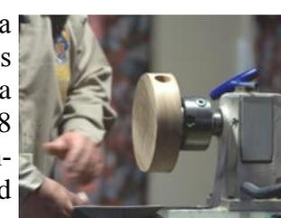
This blank was mounted on the screw chuck, trued up around the circumference and on the flat face. David then used a parting tool to take out the centre until he reached the top of the screw chuck. At the edge of this opening he made a small shoulder, to allow the lid to sit without protruding too much. He then shaped and sanded the outside of the body.
