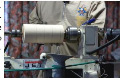
Once chucked up and trued up again, he then divided the cylinder into equal sections, two for a large cove, forming the neck of the vase, one for the bottom of the vase, and finally one designated as a waste section.
