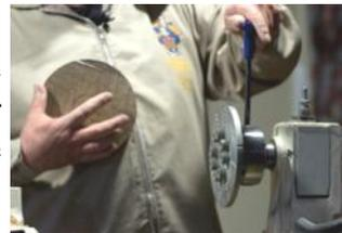
On the entire piece David demonstrated the use of cutting wax from Mylands, applied with the roughest grade of Nypad, and smoothed and polished with increasingly finer Nypads and finally with an application cloth, achieving a soft shine (not a high gloss).
