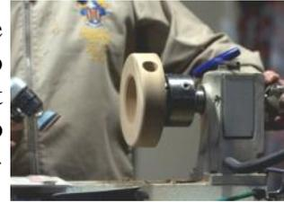
He then changed over to Cole jaws, mounted the body, trued up the face and sanded it, before taking out the rest of the centre. In other words, he now had a ring with two shoulders on both sides of the inside edge and a hole through the side into the inner opening.
