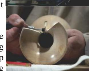
The zip is held in place with medium viscosity CA glue. David first glued in the bottom (closed) half, then went halfway up the V shape, and then glued the final bit. The zip needs to sit right at the front edge of the wood to look natural. The final bit is a few drops of glue at the back of the zipper, to ensure it doesn't work itself or any other part of the zip loose.
