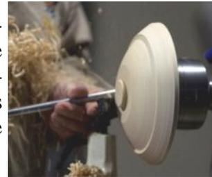
David also put a bead on the rim, about 1/2" from the edge, and then sanded the rim with the lathe stopped. Due to the eccentricity of the bowl, sanding with the lathe running is not recommended and can be dangerous.
